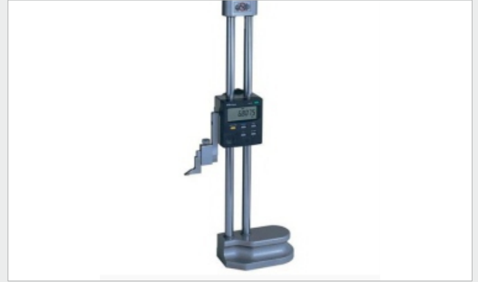
Height Gauge - 1 No.s (0-300 mm)
